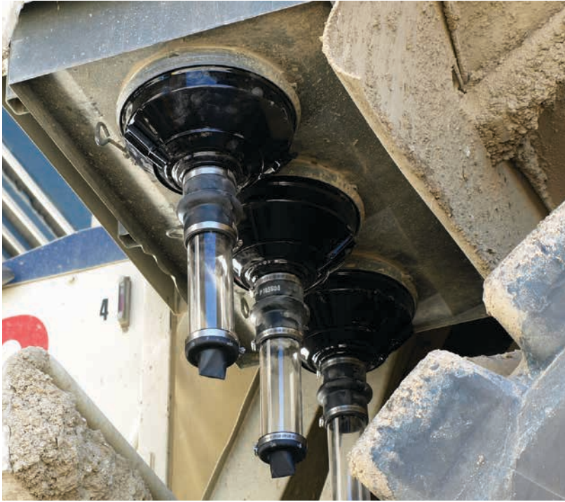
Three kits are required for S Series dual outlet models. For proper performance all dust cups must have the new Dust Dumpa installed.
