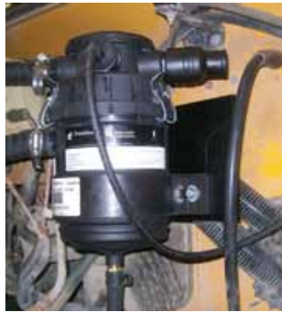
FIGURE 4 SPIRACLE SYSTEM ON A SCHOOL BUS
