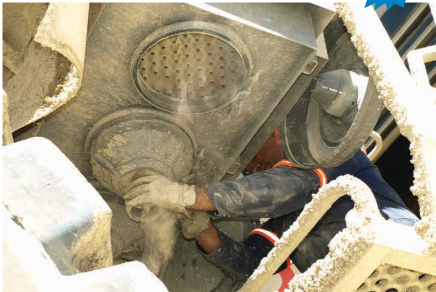
If the above maintenance practice looks familiar, adding the X006561 Dust Dumpa extension to the dust cups of the air cleaner will save you maintenance time and will minimize your employees exposure to nuisance dust during service.
